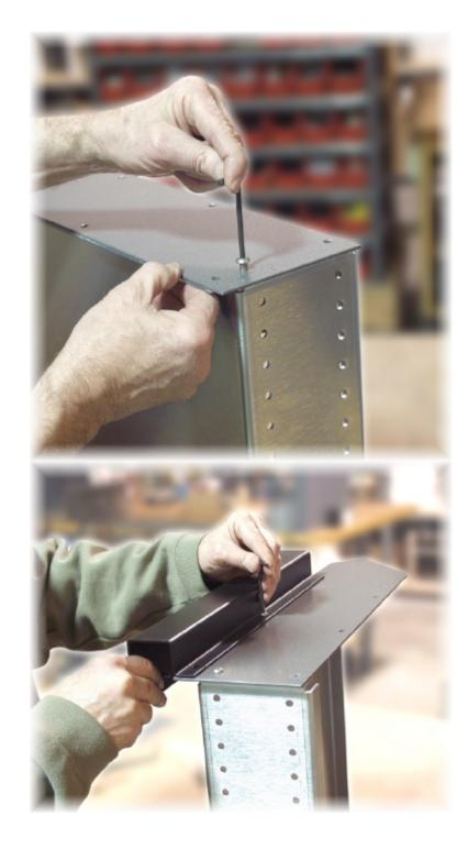
Locate one of the top rails and line up its 3 holes with the mating holes in the side cover.
