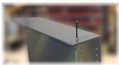
Thread one of the ¼-20 X 3/8" screws into the middle hole in the short side of panel. The is the only screw that is not used to secure the top or bottom rails.
